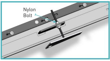
Once nylon bolt is secure, pull joint towards you and stand the joint upright.
