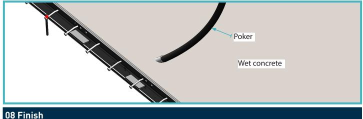
Finish concrete, flush to top of the armoured joint ensuring the rail is clearly viable.
