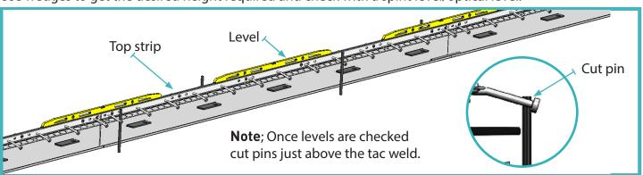
Measure the vertical and horizontal level using the top strip.
