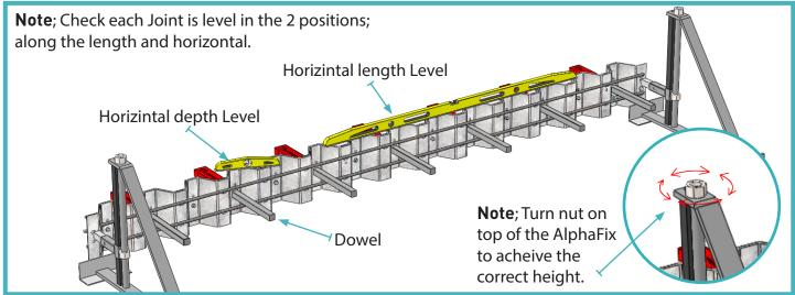
Once Joints are level hammer pins can be used for extra support.
