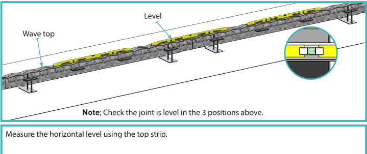
Note; Joints must be fixed at 90°. Note: Adjust the bottom nut to get the desired. height. AlphaFoot.
