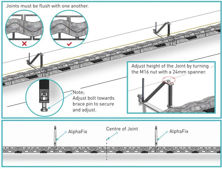
Check the level of the Joints with an optical leveler in three positions below.
