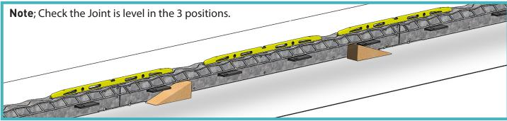
Once Joints are level hammer pins ether side of the joint and tack weld in position.
