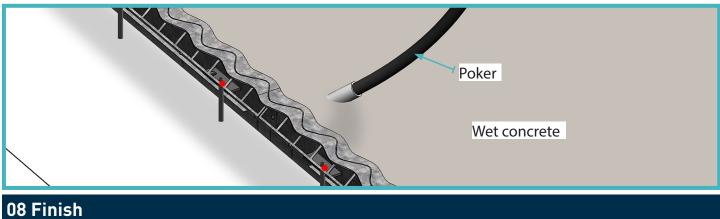
Finish concrete, flush to top of the Joint ensuring the rail is clearly visable.
