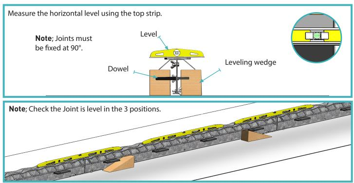
Once Joints are level hammer pins ether side of the joint and tack weld in position.
