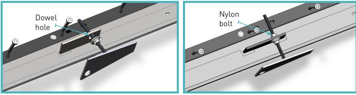
Once nylon bolt is secure, pull joint towards you and stand the Joint upright.
