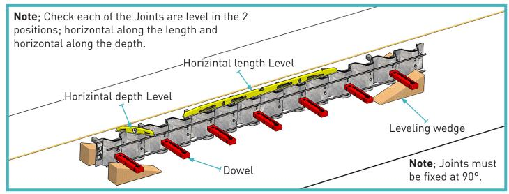
Once Joints are level hammer pins ether side of the Joint and tack weld them to the rebar.
