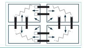
Two-way lateral movement allows free contraction as the slab cures - no cracking.
