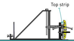
Note; Measure the vertical and horizontal level using the top strip. Level
