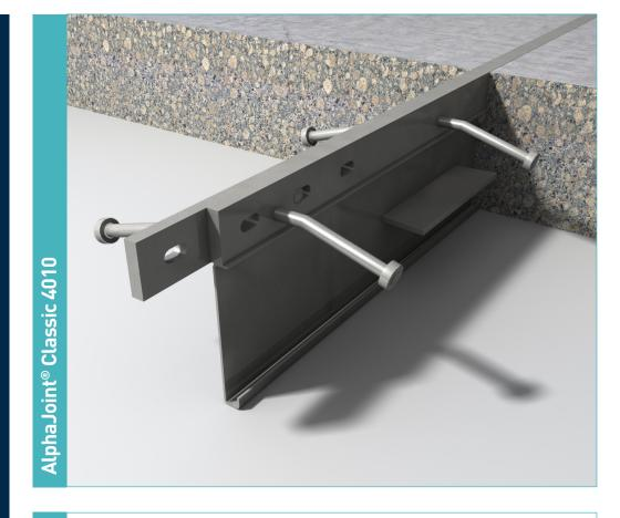
10mm wide cold drawn, square edge 10mm x 100mm shear steel\* provides joint arris armouring studs anchor AlphaJoint to concrete Frangible fixing system AlphaJoint® Classic 4010 Plate dowel sleeve to \*\*Plate dowel provides load debond dowel transfer across joint Sheet steel formwork Universal Extension \*Also available in galvanised and stainless steel to suit slab depths 150 - 200 \*\*Dowels available in thicknesses of 6mm, 8mm and 10mm
