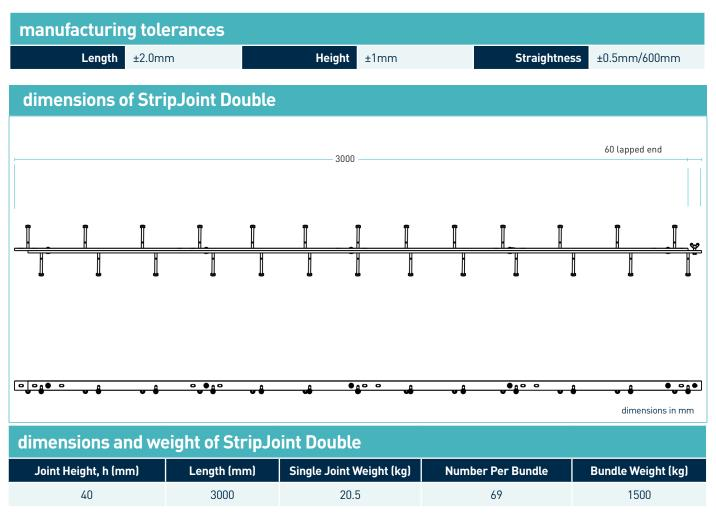
Typical height and length values shown only. Weight values shown are based on mild steel StripJoint and are approximate.
