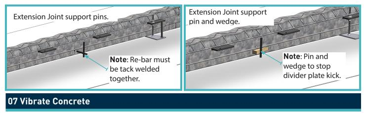
Poker vibrate along length of the joint to compacted concrete.
