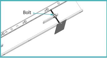
Once the steel bolt is secure, pull joint towards you and stand the Joint upright.
