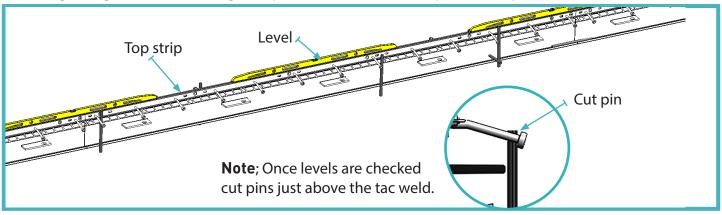
Measure the vertical and horizontal level using the top strip.
