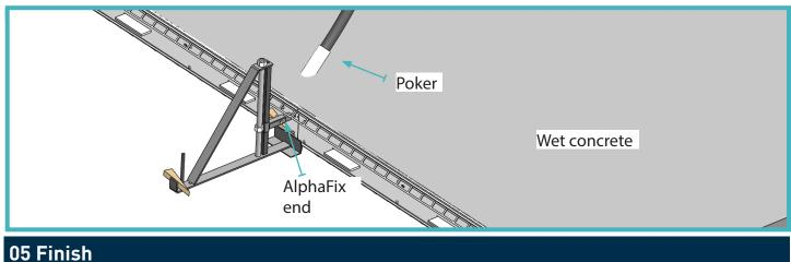
Finish concrete, flush to top of the Joint ensuring the rail is clearly visable. Before next side is cast, cut Joints support pins.
